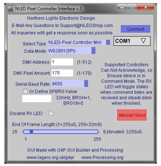
Connect to COM Port, input configuration data, start controller in Command Mode and Press "Attempt Send"
